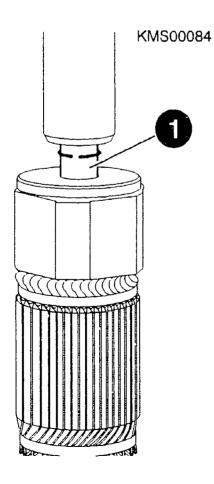
CHECKING AND REPAIRING COMPONENTS Checking armature for interturn short circuit, ground short and continuity Check for interturn short circuit with tester and test probes. Check for ground short and continuity with tester and test prods. Interturn short circuit tester: 0 986 619 110 0 986 619 114 Test prods: Ground short test voltage: 80 V Continuity test voltage: 40 V Continue: III01/1 Fig.: II28/2 16.0 KMS00085
